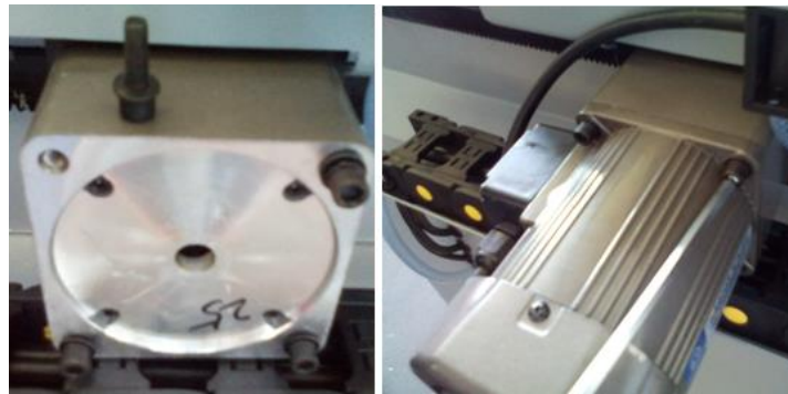
2. Travelmotor Mount with 4 screws
