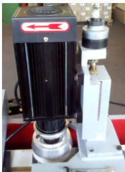
1. Mainmotor: Mount with 4 screws
