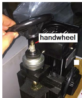
5. Handwheel: Place the handwheel and fix with the nut.
